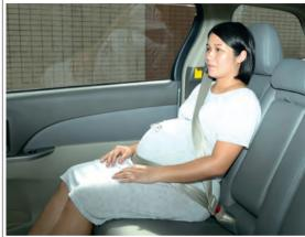
Lap belts, as well as the lap portion of a lap-shoulder belt combination, should be placed low, across the hips, under the bump and over the upper thighs. They must lie snugly over the pelvis, one of the stronger bones of the body.
