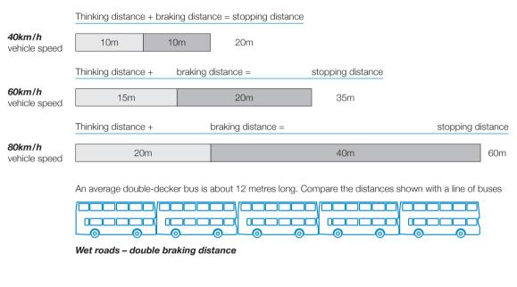
On a dry road, an alert driver with a car equipped with good brakes and tyres driving at speeds shown on the left, can stop in the distances shown on the right. These are the shortest stopping distances.
