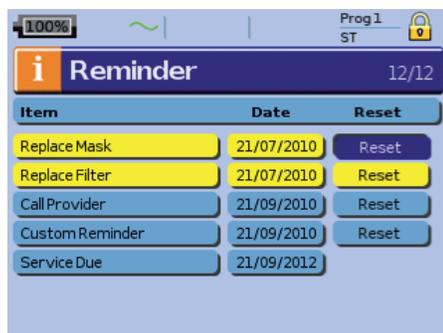
The Clinician uses the Reminders menu to alert you to specific events; for example, when to replace the mask, when to replace the filter and so on. The reminder appears in yellow as the date approaches (within 10% of the reminder period). The reminder also displays on the startup screen. You can clear a reminder message by selecting 'Reset', which clears the current reminder date to OFF, or displays the next pre-set Reminder date.
