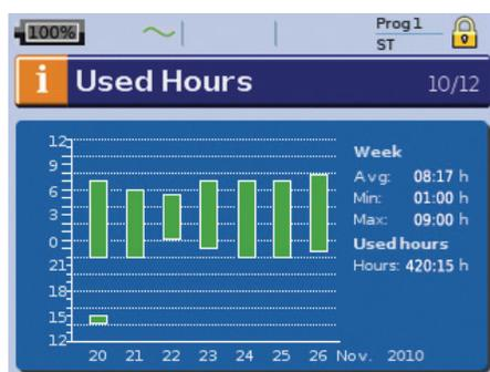
Used Hours during the last seven days of treatment are displayed in a bar graph and can be compared to the data of the last 365 days.
